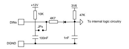
Figure 6 - Digital Input Circuit
